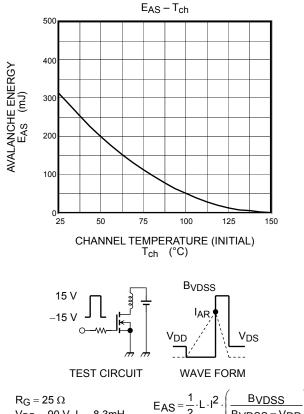
$$\begin{aligned} R_G &= 25~\Omega \\ V_{DD} &= 90~V,~L = 8.3 mH \end{aligned}$$
