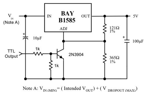
Fig.7 5V Regulator with Shutdown
