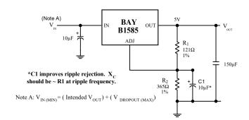
Fig. 6 Improving Ripple Rejection
