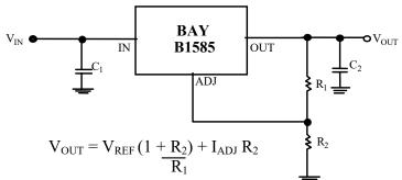
Fig 5. Typical Adjustable Regulator
