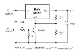
Fig.7 5V Regulator with Shutdown
