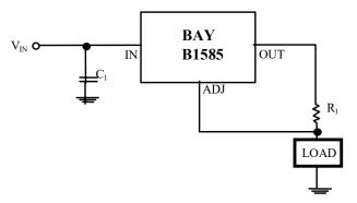
Fig.4 5A Current Output Regulator
