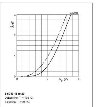
Fig.15 Forward current as a function of forward voltage; maximum values.
