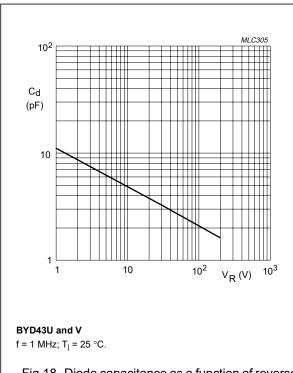
Fig.18 Diode capacitance as a function of reverse voltage; typical values.
