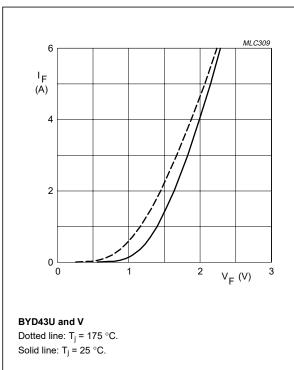
Fig.14 Forward current as a function of forward voltage; maximum values.
