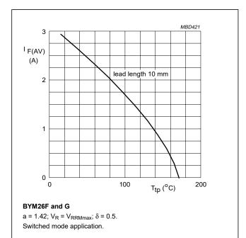
Fig.3 Maximum average forward current as a function of tie-point temperature (including losses due to reverse leakage).
