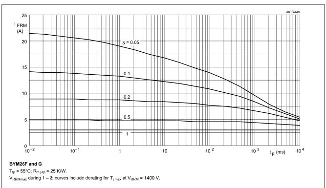
Fig.7 Maximum repetitive peak forward current as a function of pulse time (square pulse) and duty factor.
