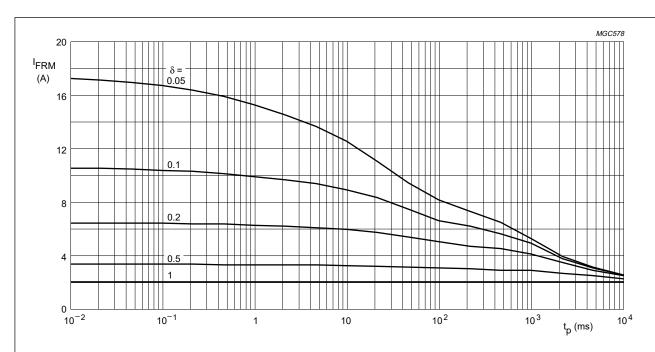
$T_{tp}$  = 65 °C;  $R_{th j-tp}$  = 46 K/W.
