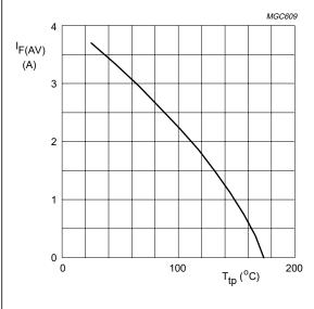
a = 1.42;  $V_R = V_{RRMmax}$ ;  $\delta$  = 0.5. Switched mode application.
