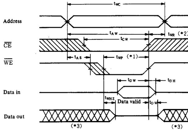
Write Cycle (2):  $\overline{CE}$  Control [ $\overline{OE}=V_{IL}$ ]
