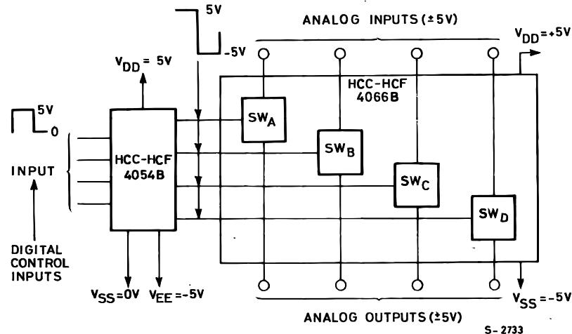
**TYPICAL APPLICATIONS (4-CHANNEL PAM MULTIPLEXER SYSTEM DIAGRAM)**
