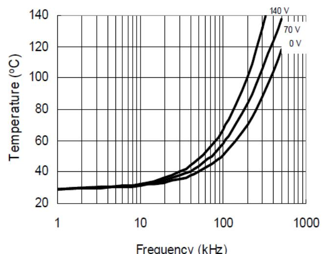
Figure 24. IRS2186 vs. Frequency (IRFPE50)
