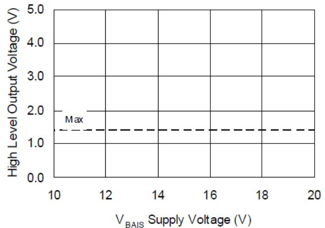
**Figure 10B. High Level Output Voltage vs. Supply Voltage ( $\text{I}_\text{o} = 0\text{mA}$ )**
