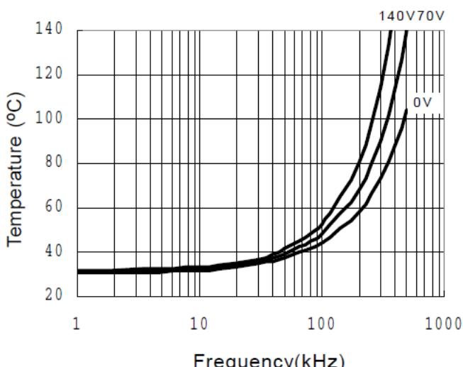
Figure 31. IRS2186S vs. Frequency (IRFBC40)
