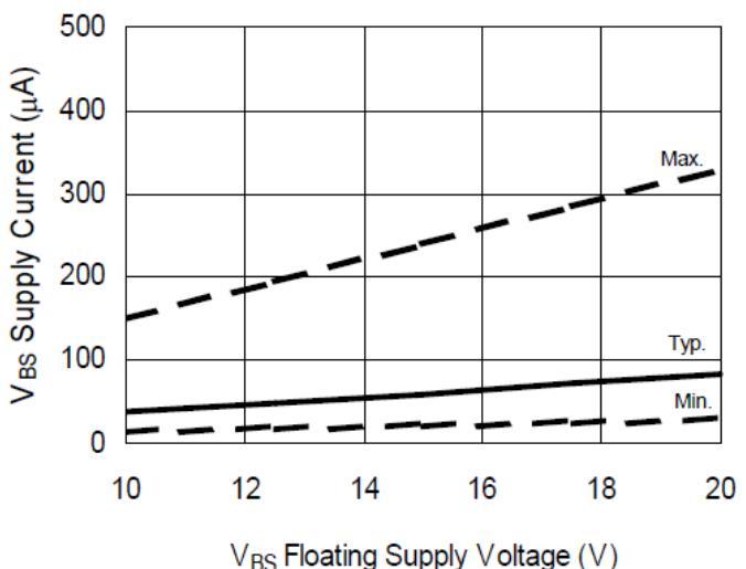
Figure 13B. V<sub>BS</sub> Supply Current vs. V<sub>BS</sub> Floating Supply Voltage
