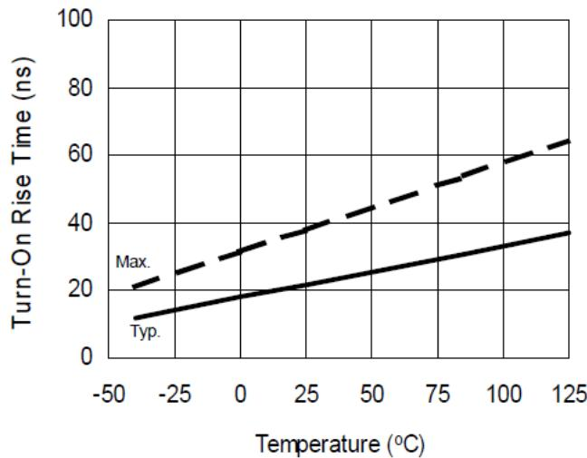
Figure 6A. Turn-On Rise Time vs. Temperature
