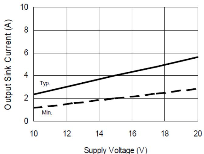
Figure 10B. Output Sink Current vs. Supply Voltage
