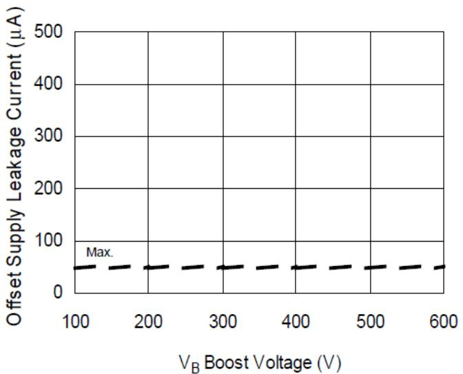
Figure 12B. Offset Supply Leakage Current vs. V<sub>B</sub> Boost Voltage
