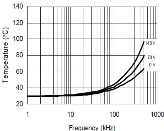
Figure 35. IRS21864S vs. Frequency (IRFBC40)
