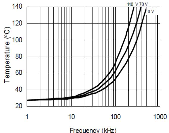
Figure 36. IRS21864S vs. Frequency (IRFPE50)
