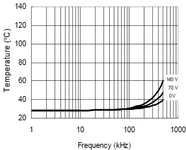
Figure 33. IRS21864S vs. Frequency (IRFBC20)
