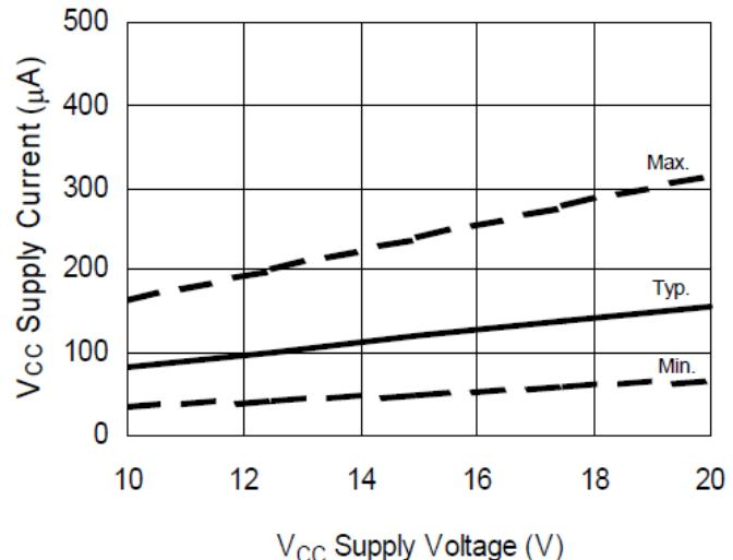
Figure 14B. V<sub>CC</sub> Supply Current vs. Supply Voltage
