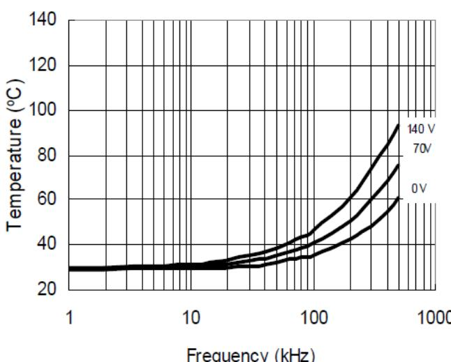
Figure 23. IRS2186 vs. Frequency (IRFBC40)
