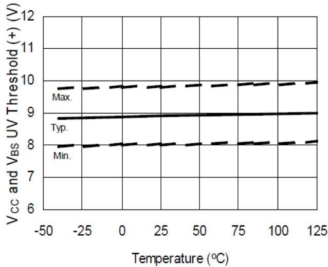
Figure 17.  $V_{\text{CC}}$  and  $V_{\text{BS}}$  Undervoltage Threshold (+) vs. Temperature
