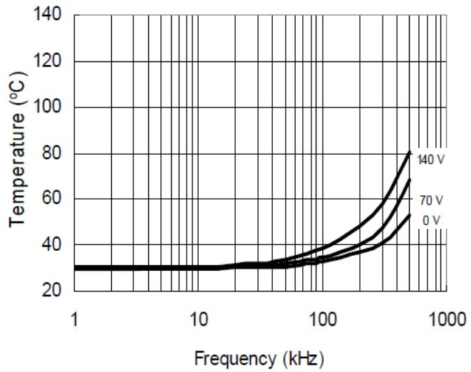
Figure 34. IRS21864S vs. Frequency (IRFBC30)
