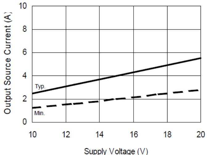
Figure 19B. Output Source Current vs. Supply Voltage
