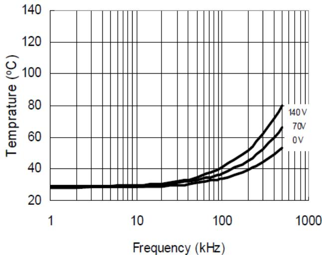
Figure 21. IRS2186 vs. Frequency (IRFBC20)
