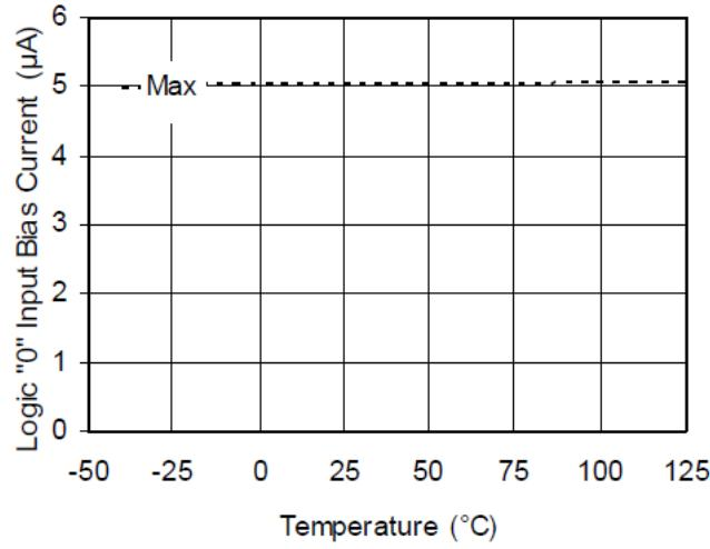
Figure 16A. Logic "0" Input Bias Current vs. Temperature
