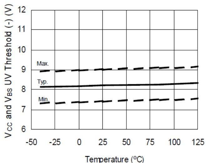
Figure 18.  $V_{\text{CC}}$  and  $V_{\text{BS}}$  Undervoltage Threshold (-) vs. Temperature
