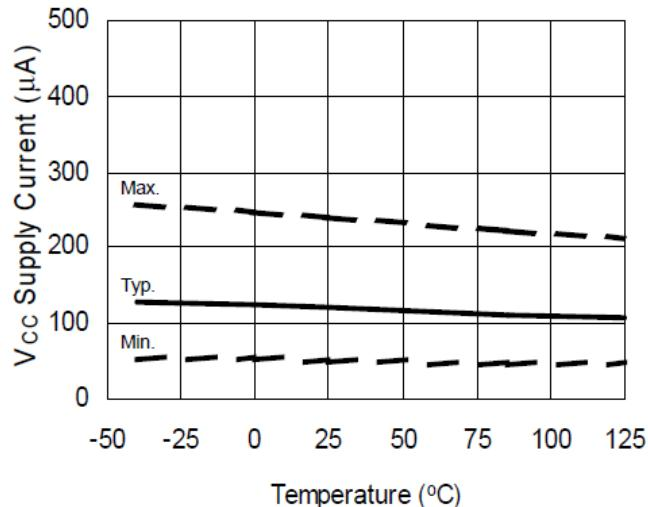
Figure 14A. V<sub>CC</sub> Supply Current vs. Temperature
