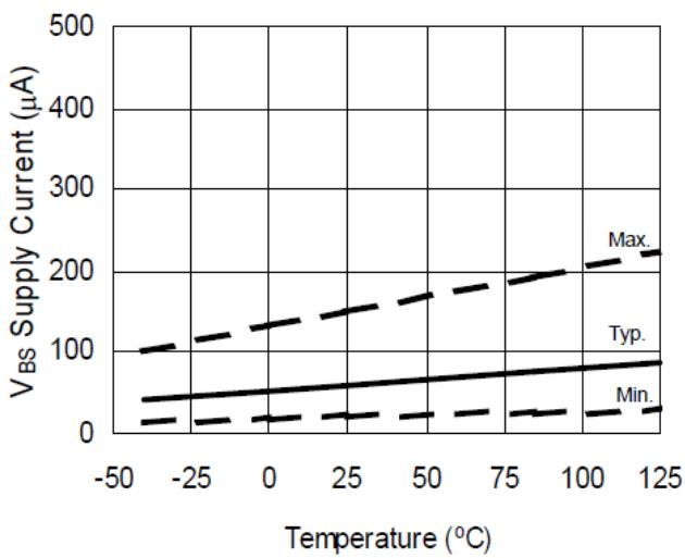
Figure 13A. V<sub>BS</sub> Supply Current vs. Temperature
