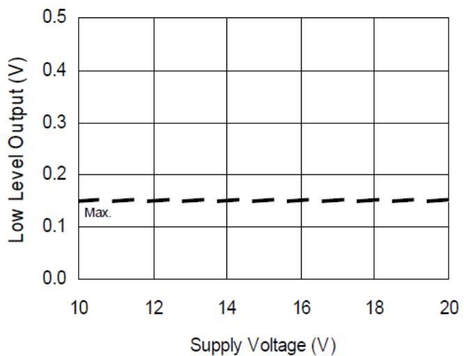
**Figure 11B. Low Level Output vs. Supply Voltage**
