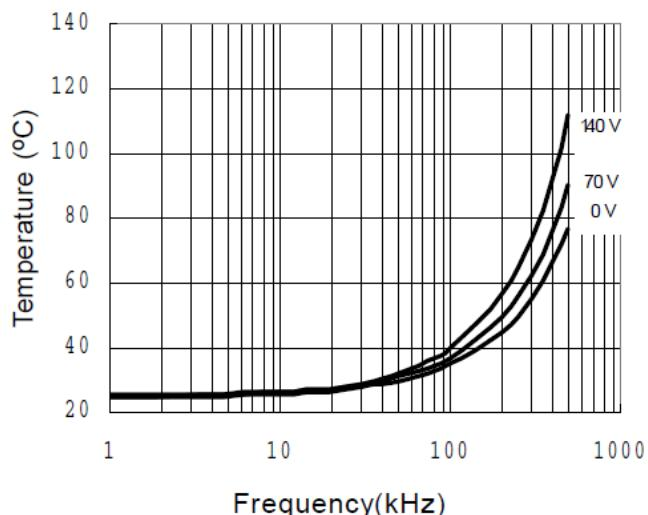
Figure 30. IRS2186S vs. Frequency (IRFBC30)
