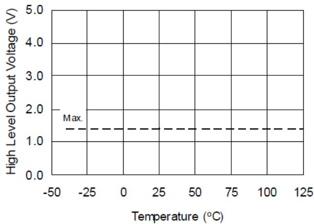
**Figure 10A. High Level Output Voltage vs. Temperature ( $\text{I}_\text{o} = 0\text{mA}$ )**
