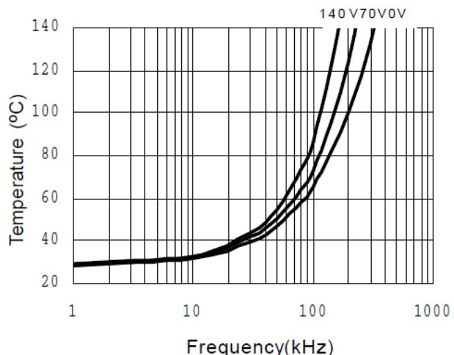
Figure 32. IRS2186S vs. Frequency (IRFPE50)
