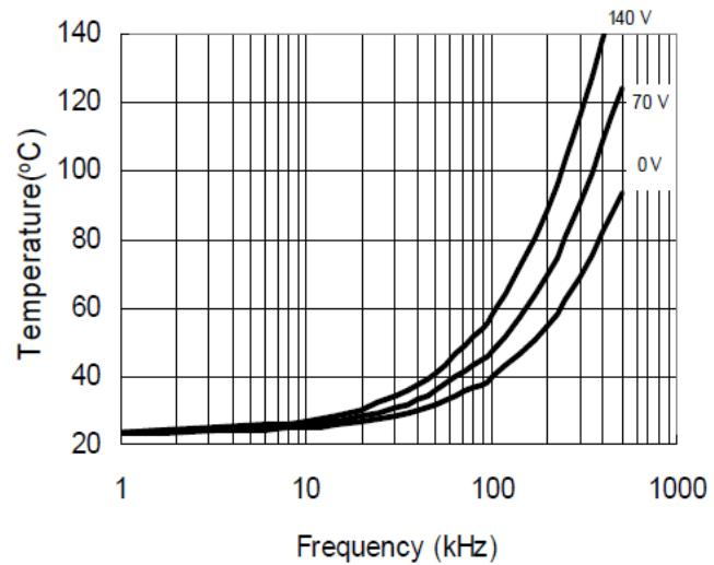
**Figure 28. IRS21864 vs. Frequency (IRFPE50)**
