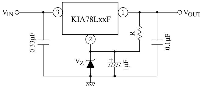
$$V_{OUT} = V_Z + V_{OUT} (\text{of IC})$$
