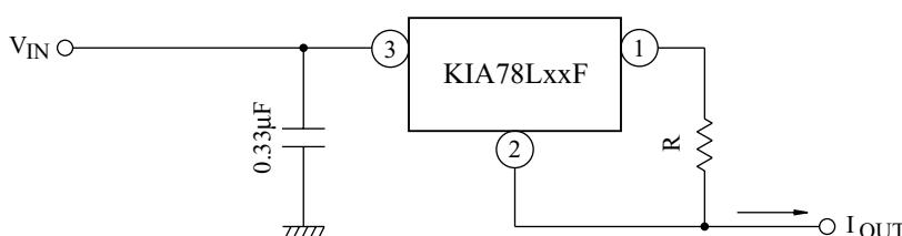
$$I_{OUT} = \frac{V_{OUT}}{R} + I_B$$
