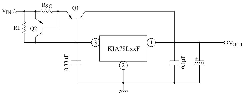
$$R_{SC} = \frac{V_{BE2}}{I_{SC}}$$
