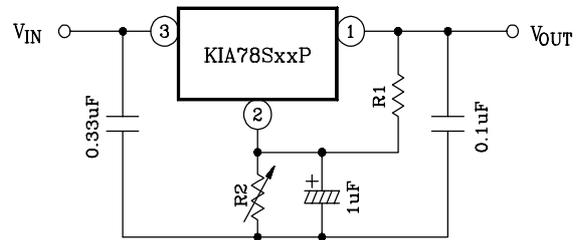
$$V_{OUT} = R_2 \left( I_B + \frac{V_{OUT} \text{ (of IC)}}{R_1} \right) + V_{OUT} \text{ (of IC)}$$
