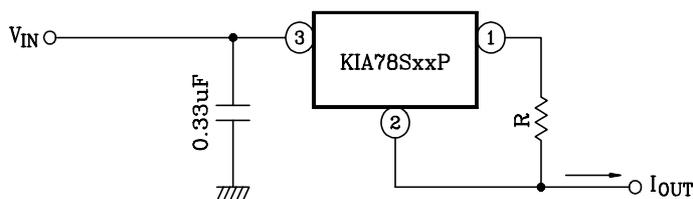
$$I_{OUT} = \frac{V_{OUT}}{R} + I_B$$
