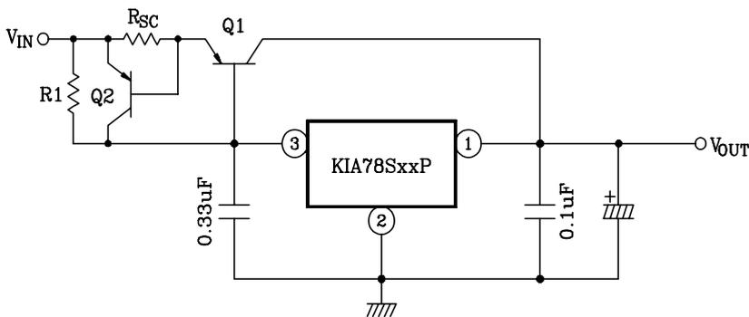
$$R_{SC} = \frac{V_{BE2}}{I_{SC}}$$
