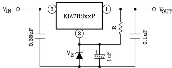
$$V_{OUT} = V_Z + V_{OUT} \text{ (of IC)}$$
