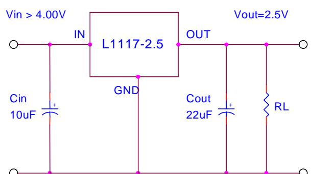
**Basic Fixed Output Regulator Circuit**
