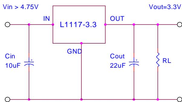
**Basic Fixed Output Regulator Circuit**
