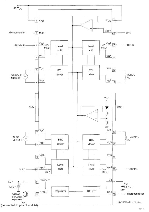
Note: Use a delay capacitor (Cd) whose capacitance does not change much according to the temperature.
