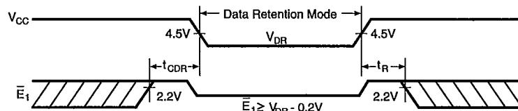
LOW  $V_{CC}$  DATA RETENTION WAVEFORM (2) ( $E_2$  Controlled)
