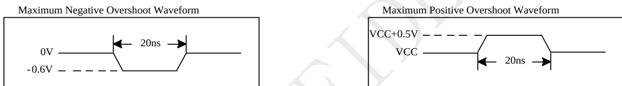
Figure 5-1 Maximum Overshoot Waveform
