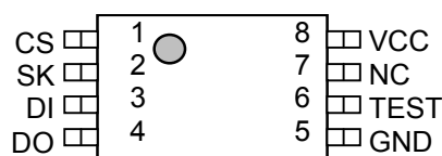
8-Pin TSSOP Top view
