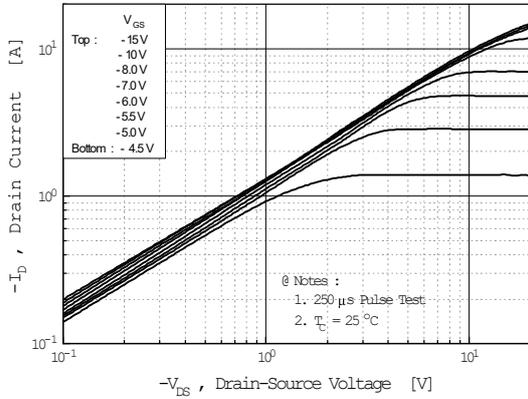
**Fig 2. Transfer Characteristics**
