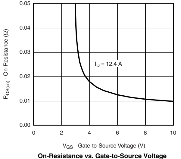
On-Resistance vs. Gate-to-Source Voltage
