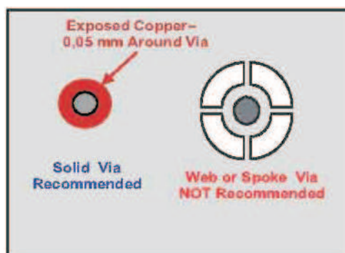
Figure 27. Thermal Via Connection at the Bottom Layer
