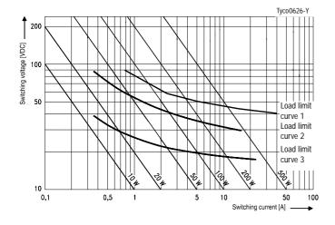
Load limit curve 1  $\stackrel{\triangle}{=}$  safe shutdown, connected as form X, load on pin 5 and 7
